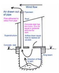
Figure 2-4: Effect of venting a pit toilet
