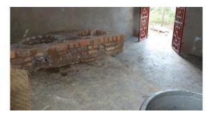
The stoves vent to external chimneys so the cook does not have to breathe in smoke from the fires.
